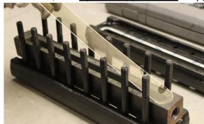
9. Locate the glass centrally in the chamber seat and cover to avoid glass-to-metal contact at the ends or sides. Using cardboard from the glass kit box, cut strips to use as spacers to locate the new glass in place on top of the gasket and mica in the chamber. Remove the cardboard once the glass is located properly (this is best done with the gage lying flat on a bench).
