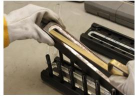
5. Thoroughly inspect all chamber gasket surface seating areas. Remove any pitting damage, steam cuts, gouges or scars on a milling machine. Gasket surface flatness must be maintained within 0.002" (0.05mm). The minimum material thickness dimension shown in Figure A (page 14) must also be maintained. On most Jerguson
