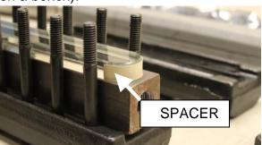
10. Apply Molykote® or a similar molybdenum disulfide lubricant to the bolt threads and nut seating surface. If the gage has spring washers, reference Figure B (below) for proper orientation of the washer stacks.
