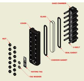
Jerguson gages use molded borosilicate glass, tempered to increase bending resistance. The glass has a low coefficient of expansion, is more resistant to thermal shock than other glass and is much stronger in compression than in tension. However, as with any glass, care should still be taken to avoid imposing any bending or local stresses or direct glass to metal contact.
